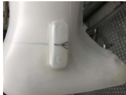
Fig. 4 Note the hole in the dummy through the plastic and trim line
